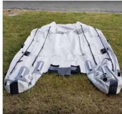
2. Locate the inflator valve at the rear of the hulls and inflate to 3 psi with the included hand pump or optional electric pump. Don't forget to activate the check valve in the inflation valve by pressing down on the centre pin and turning it ¼ turn in either direction. If the check valve is popped up, it won't let any air escape.
