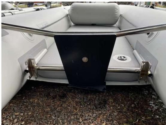
4. From the front, insert the upper transom bar into the upper set of tubes on the boat hulls. The stainless tab should be facing down when insert properly.
